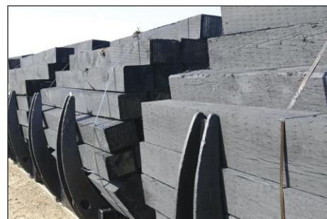
And they treat a lot. Note the cleanliness of these freshly treated ties!
