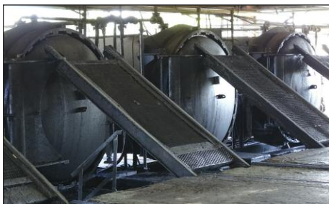
Their four 8 ft. x 155 ft. cylinders are the workhorses for this operation.
